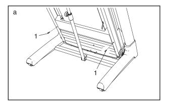
Lower the treadmill (see HOW TO LOWER THE TREADMILL FOR USE on page 25). Remove the four indicated #8 x 3/4" Screws (1), and remove the Motor Hood (75).
